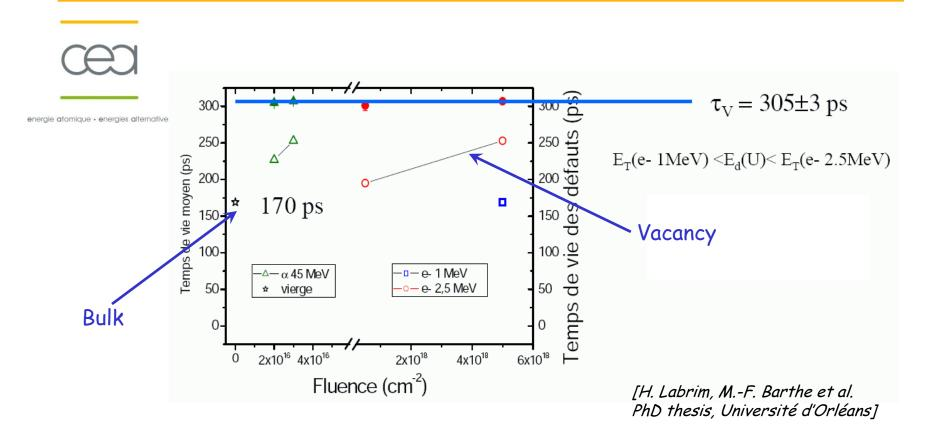
Calculations validate the assumption that irradiated UO<sub>2</sub> samples contain Shottky defects
